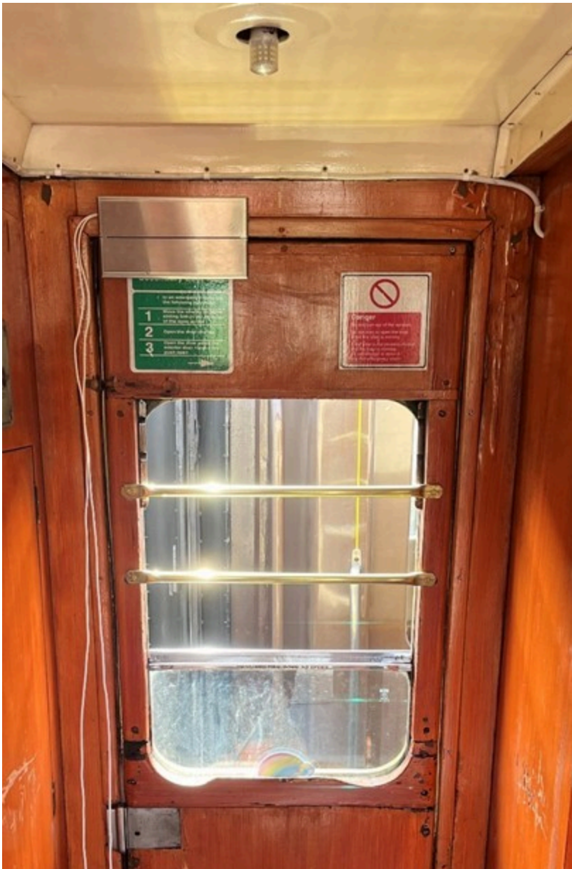
Photo: Vintage trains fitment of a central locked door bolt
