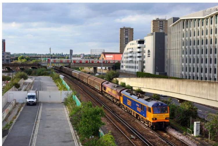
A Class 92 dual voltage locomotive approaching Shepherds Bush southbound on the West London line. Source: Railway Centre
