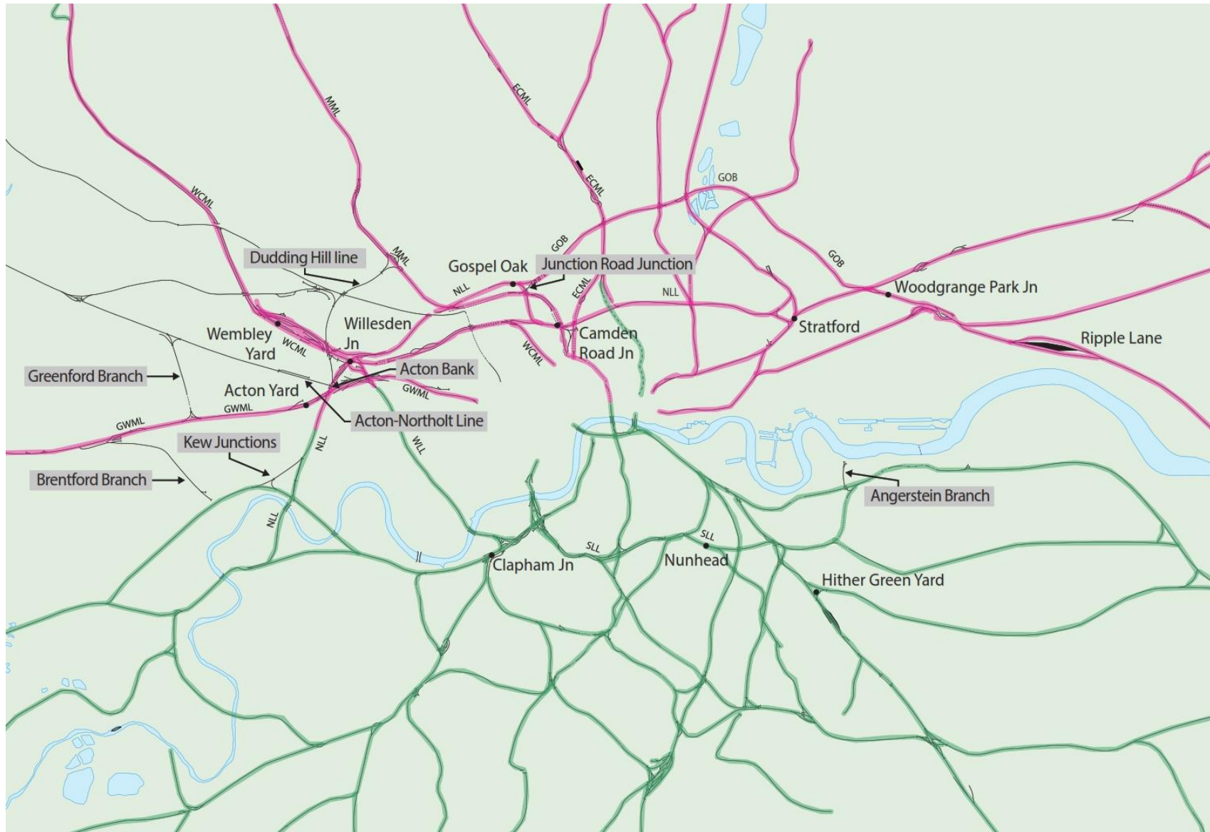
Figure 15: Railway electrification. The pink lines highlight 25 kV AC, the green lines highlight 750 V DC and the grey boxes highlight lines without electric traction capability.
