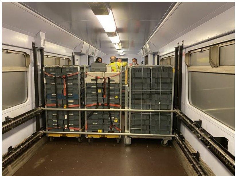
Train interior following conversion to accommodate roll cages.
