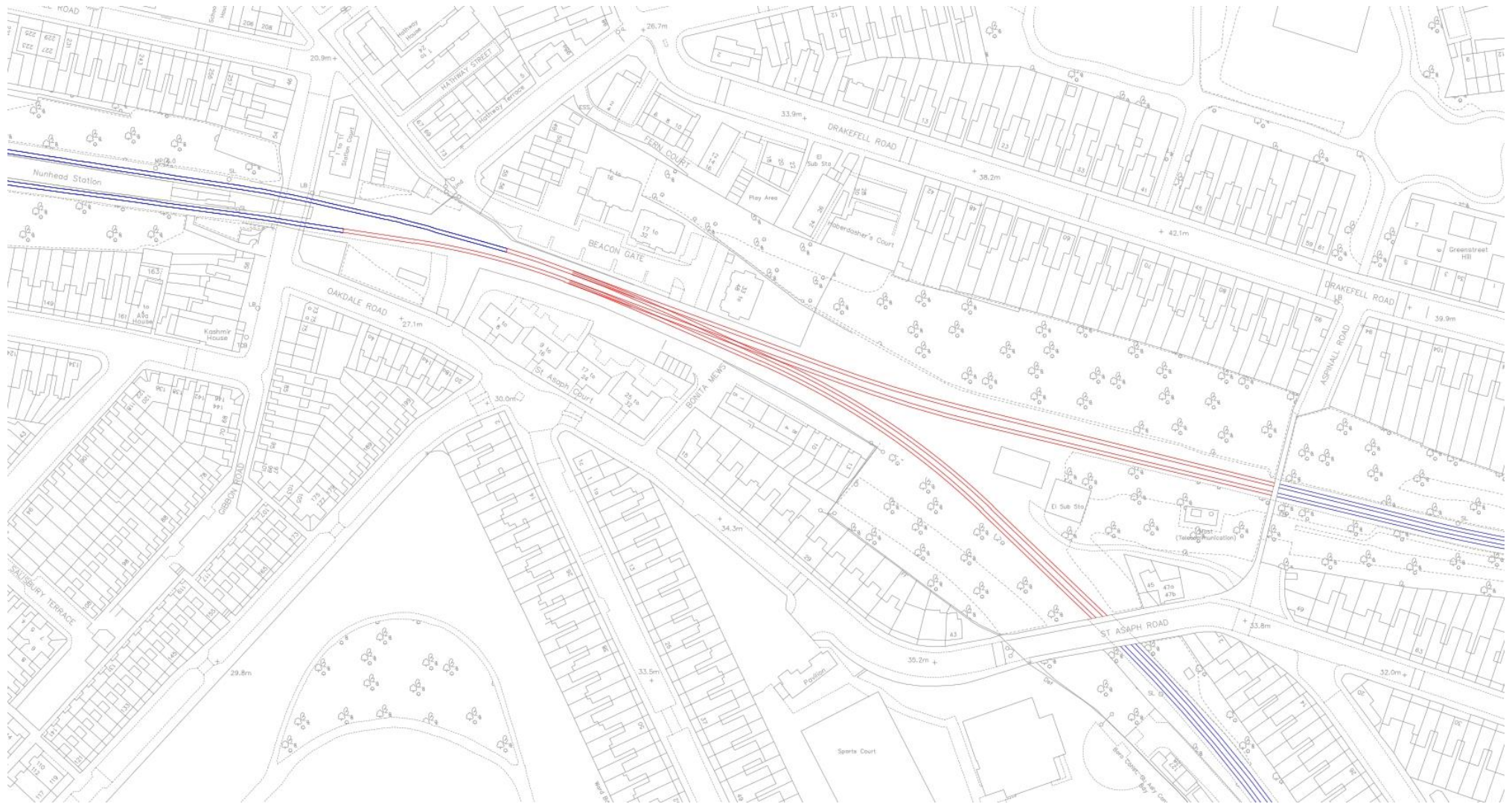
Figure 34: Detail from initial conceptual design sketch of the proposed Nunhead Junction Improvement scheme (see Appendix A for full sketch)
