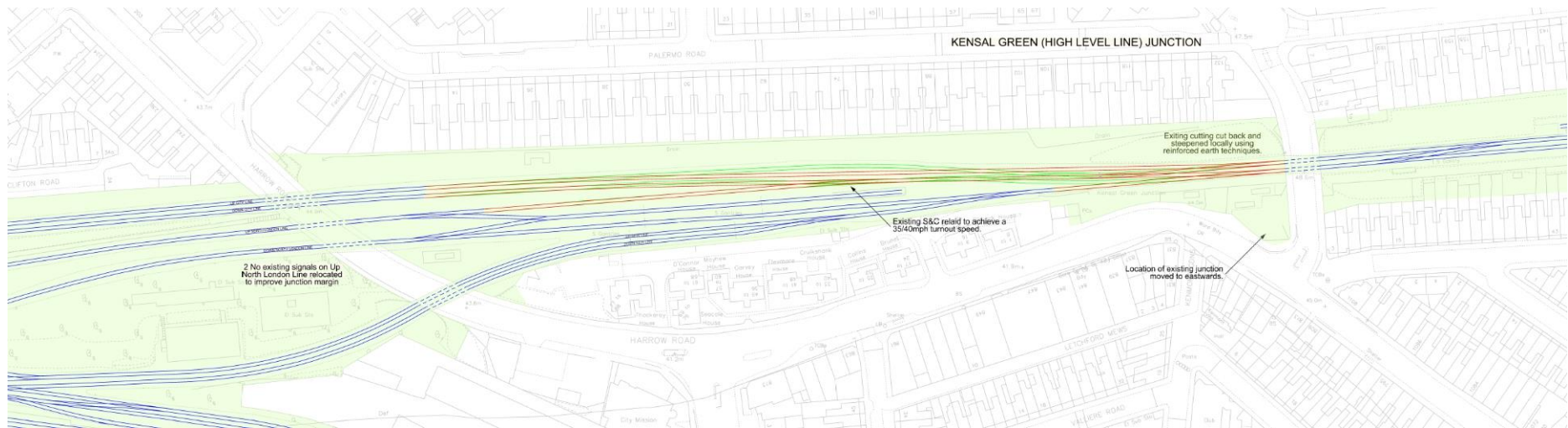
Figure 19: Detail from conceptual design sketch of the proposed Kensal Green Junction Improvement scheme (see Appendix A for full sketch)
