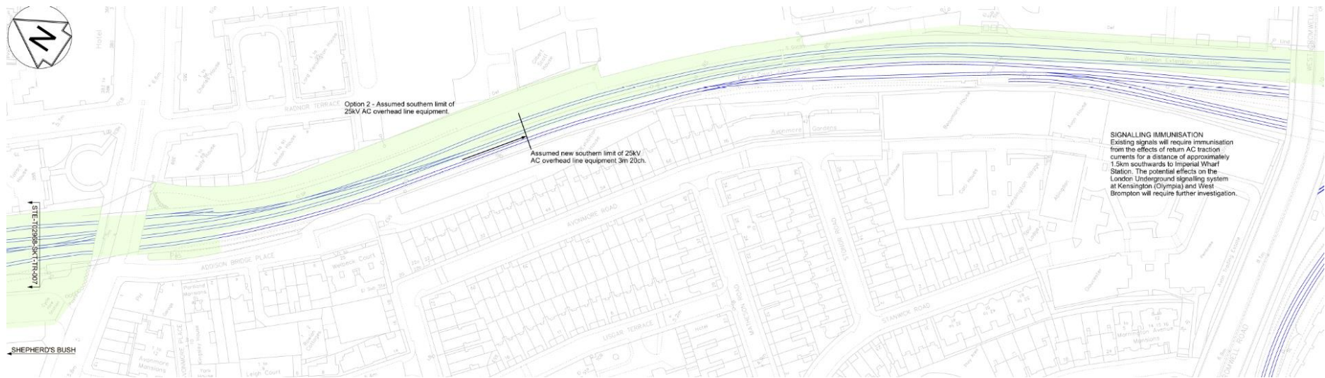
Figure 28: Detail from conceptual design sketch of the proposed relocation of the West London Line AC/DC changeover – Option 2 to Kensington Olympia (see Appendix A for full sketch)
