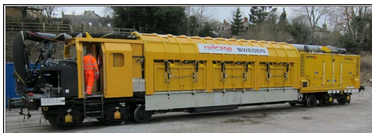
Fig.10 RailVac. The machine has an on board storage for 15 cubic metres of material
