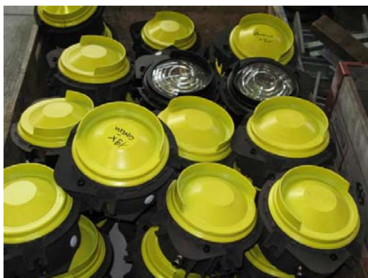
Refurbished signal heads
