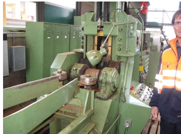
Roller press for straightening the rails
