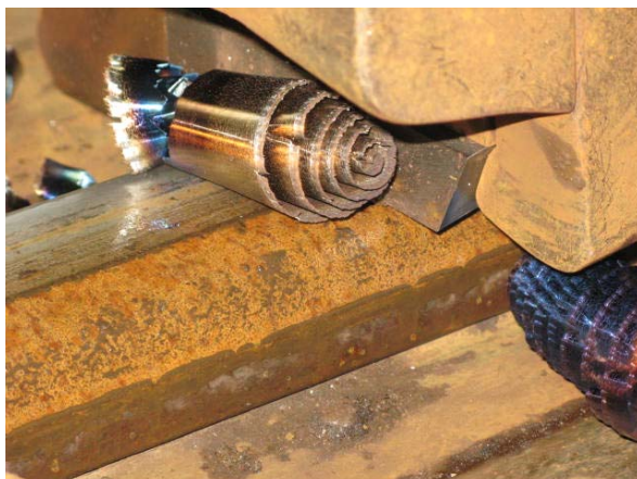
Rail profiling through planing
