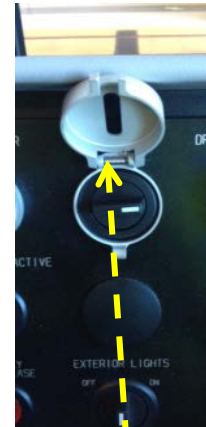
Switch in override position
